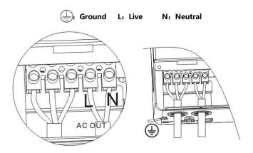
**Note:** The grounding wire shall be as thick as possible (cross-sectional area is not less than 4mm<sup>2</sup>). The grounding point shall be as close as possible to the hybrid solar charge inverter. The shorter the grounding wire, the better.
